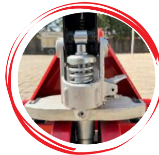
Fork Lowering: Hand control and Foot pedal
