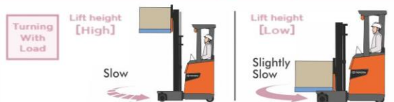
Vehicle speed adjusted accordingly to turning radius, load weight and lift height.
