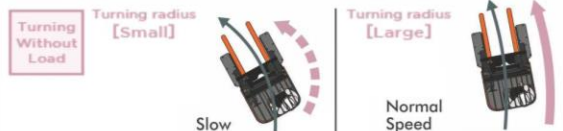
Vehicle speed adjusted accordingly to turning radius
